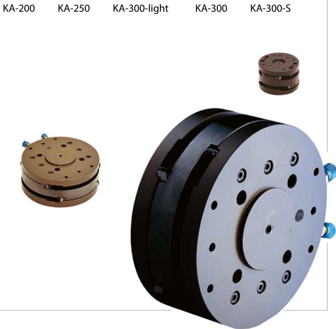
The maximum allowable moment is the decisive parameter for the selection of lateral alignment devices. Additional part-picking or placing forces which can work as moment loads on the guides must be taken into account. The maximally arising moment determines itself from the payload of gripper and part, the procedure movement of the robot and from possibly additionally influencing forces in the withdrawal and
